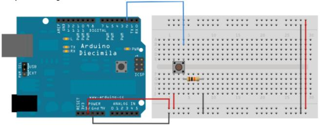
Now we will write the program that reads a digital input through pin 2, prints the result to a serial monitor (which monitors any input coming in).
